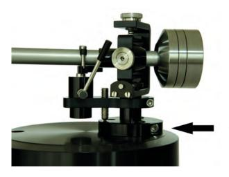
Now adjust the vertical tracking angle (VTA). It's usually best to start with the tonearm tube parallel to the LP when the tonearm is lowered onto the record surface. (Proper Stylus force must be applied before obtaining parallel adjustment.) This usually is close to proper VTA and provides a good reference point.
