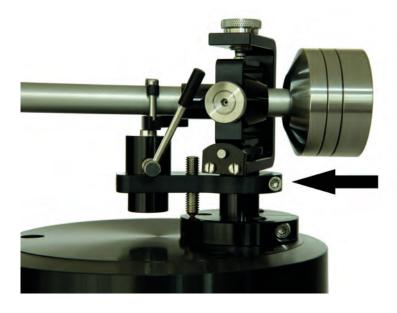
The tonearm cueing mechanism of the **10.5** and **12.1** can be heightadjusted by loosening the screw at the back of the plate that holds the cueing device and raising or lowering it.
