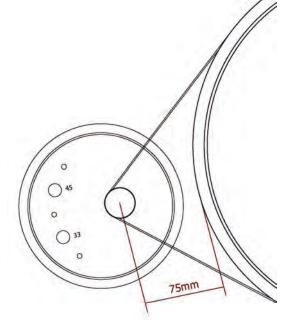
The motor can be placed in any free position around the turntable, the <u>optimal distance</u> between the platter rim and the centre of the motor pulley is **7,5cm**.
