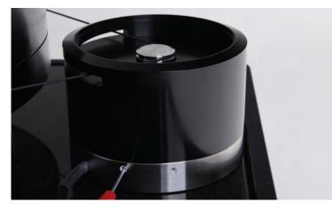
clockwise increases the speed, anti-clockwise decreases the speed. The left trim pot (viewed from the front of the turntable) is for the adjustment of 33 RPM and the right trim pot for 45 RPM. When viewed from the Speed Selector Switch, the trim pot for 33 RPM is on the same side as the 33 RPM button and the 45 RPM trim pot is on the same side as the 45 RPM button.
