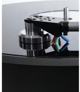
When looking at the front of the tool, it should be level on the platter surface. If there is a gap on one side, loosen the screw on the underside of the headshell to turn it until it's level, tighten the screw and check again.
