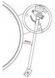
the screw in the mounting socket is loosened, the tonearm tube should have a distance to the platter of approx.. 3cm where it's closest to the platter to allow optimal antiskating.
