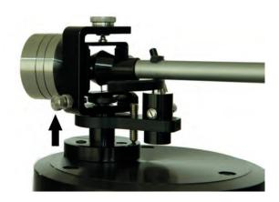
Antiskating adjustments only make sense after azimuth, HTA and VTA have been set correctly. If the desired antiskating force exceeds the maximum magnetic force it is likely that one or more of the other settings are incorrect. Please note that setting the antiskating force could also slightly change the HTA.
