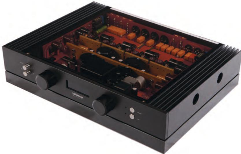
A line stage has three duties. First, it switches the various sources. Second, it controls the playback volume. And third, it conditions the signal in such a manner that even long runs of cable between line stage and power amp will not have an influence on the sound.
