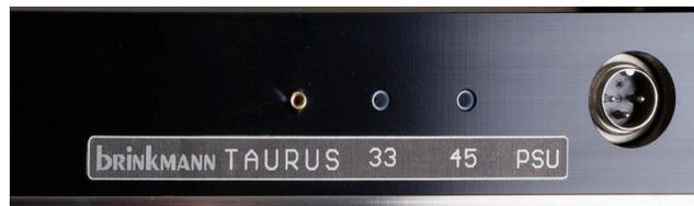
There are 2 holes located at the back of the Taurus chassis marked with “33” and “45”. They give access to the trim pots for the speed adjustment. The screwdriver included in the tool kit fits the trim pots: turning clockwise increases the speed, anti-clockwise decreases the speed.
