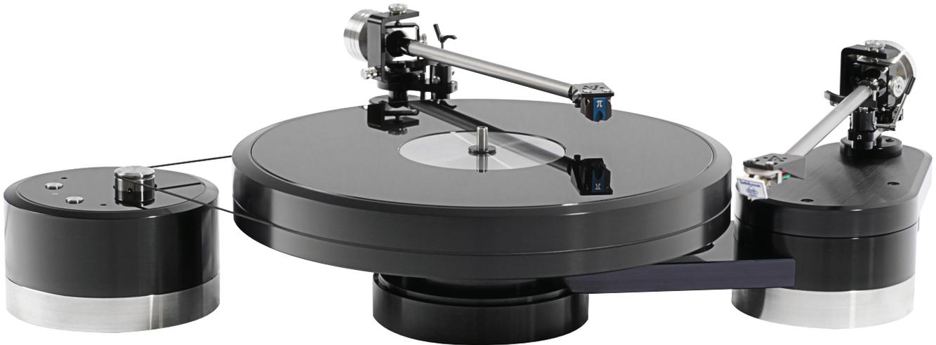
The **Spyder** turntable can be outfitted with 1 to 4 tonearms. Additional jigs with tonearm pods can be added, removed or exchanged any time. This arrangement allows a maximum of versatility and is one of the most significant design innovations of the Spyder. Unlike the Balance, which must be ordered as either a 1-arm or 2-arm turntable, any Spyder can accommodate up to four tonearms, the number of arms increasing or decreasing at the owner's whim.
