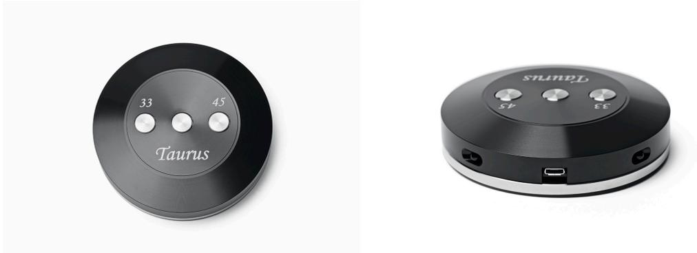
The wireless remote can be charged with a USB charger (5V) using the USB cable in the Tool kit. The battery lasts more than 10.000 on/off cycles, so charging should only be necessary after a couple of years. There is no indicator showing if the remote is fully charged. For charging, just leave remote connected to the charger overnight (8 hours). There is no indicator showing the remote is fully charged.
