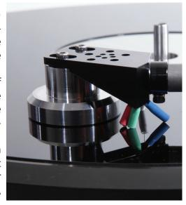
loosen the screw on the underside of the headshell to turn it until it's level, tighten the screw and check again.
