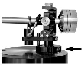
To change the VTA, loosen the screw in the mounting socket of the tonearm, now the height can be changed with the height adjustment screw. Turn clockwise to raise the back of the tonearm (at the pivot) and counterclockwise to lower it. You might be needed to push the tonearm down gently when lowering the VTA.
