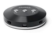
The wireless remote can be charged with a USB charger (5V) using the USB cable in the Tool kit. The battery lasts more than 10.000 on/off cycles, so charging should only be necessary after a couple of years. There is no indicator showing if the remote is fully charged. For charging, just leave remote connected to the charger overnight (8 hours). There is no indicator showing the remote is fully charged.
