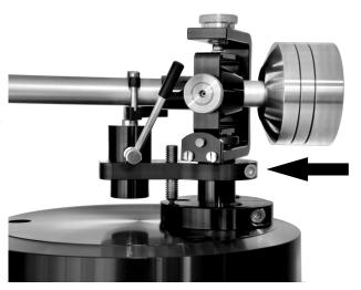
the LP instead of hitting the groove, then cleaning the rubber in the tonearm rest of the cueing with alcohol might help. The rubber holds the tonearm stable while being lowered and might fail when it's greasy.
