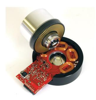
The traditional direct drive technology wasn't without problems, start-up times of less than 1 second necessitated high torque motors, which designers achieved by using motors with 32 and more poles. The penalty they paid were heavy cogging effects accompanied by high wow & flutter numbers. The cure was found in quartz locked motors and phase locked regulators; which corrected for any deviations from their preset with an iron fist.
